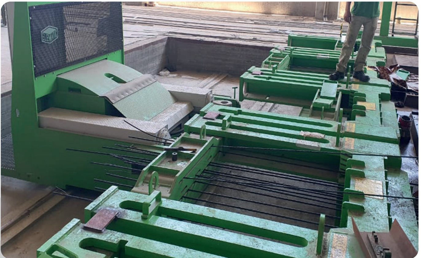
Cable strands stressing machine
