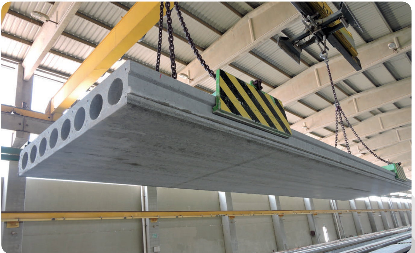
Hollow Core section after cutting
