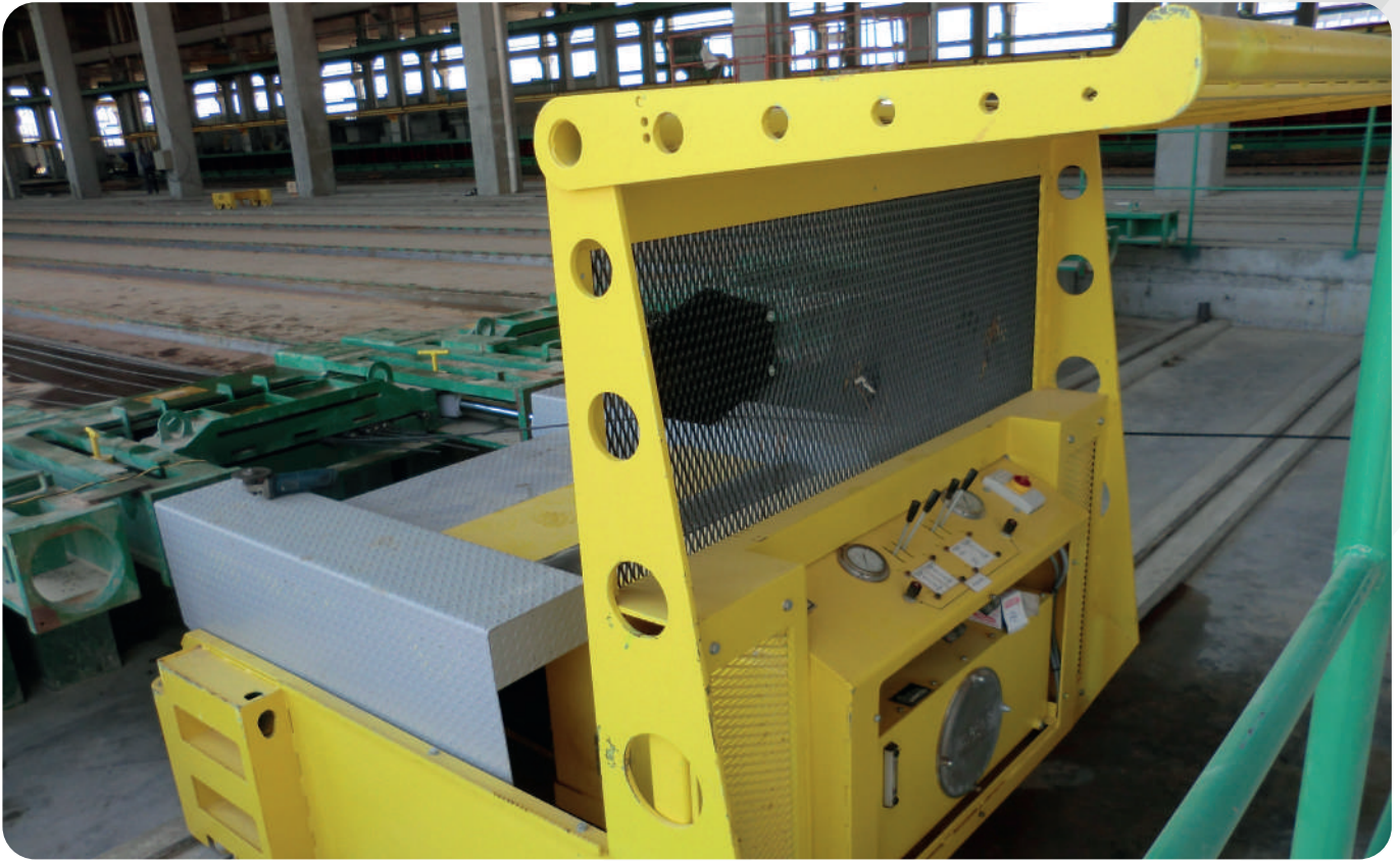
Cable strands stressing machine
